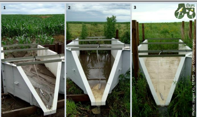
These flumes measure surface water movement and soil, nitrogen and phosphorus export from the STRIPS experiment sites at the Neal Smith National Wildlife Refuge. Compare the transport of these resources from: 1) a 100% no-till corn crop field, 2) a 90% corn crop field treated with a 10% prairie strip, and 3) a 100% prairie. These pictures were all taken after the same 4" rain event in June, 2008.
